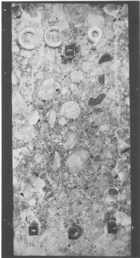
Figure 3 The pattern of surface cracking is visualized by means of the filtered particle method [28–30]. The surface crack pattern of a specimen loaded up to level 9 is shown at the left. Further, the cracks visible with the unaided eye are copied. Two of the patterns are presented below, the left one corresponding to the zero-loading stage and the right one to loading stage 9, at which the test was stopped (see Fig. 4). The uniaxial compressive stress equalled 32\text{Nmm}^{-2} at that stage.
